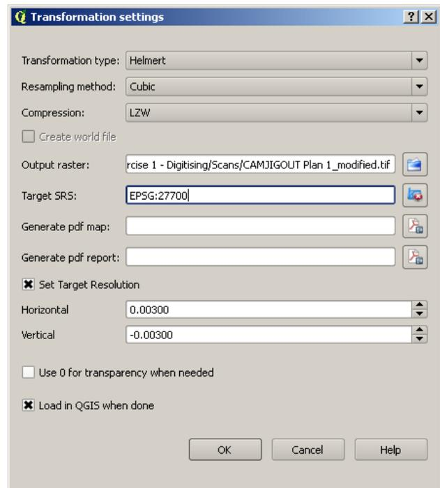
In practice you would use a GPS or theodolite in order to accurately locate your site's drawing grid points. Here we are using an arbitrary grid, but it is in metres so all digitised features will be to scale.
